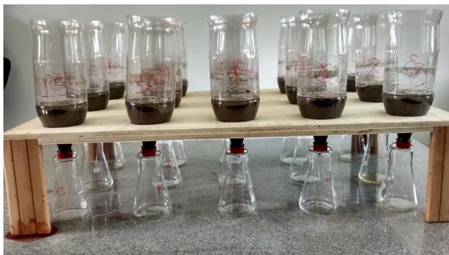
Figura 2. Lavagem do solo do PIS, com diferentes doses de gesso agrícola Figure 2. Washing of IPS soil, with different doses of agricultural gypsum
