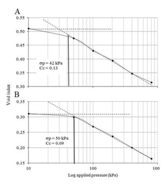
**Figure 2.** Empty index versus decimal logarithm of the applied pressure in the conventional tillage (A) and no-tillage (B).
