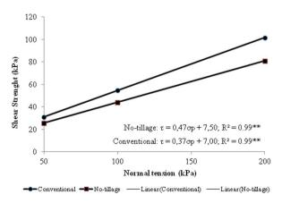
Figure 4. Shear stronght ( $\tau$ ) *versus* normal tension ( $\sigma$ p) of the soil in the conventional tillage and no-tillage.
