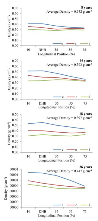
**Figure 3.** *Pinus taeda* wood density for old age, longitudinal and radial position (e = external; c = central; i = internal).
