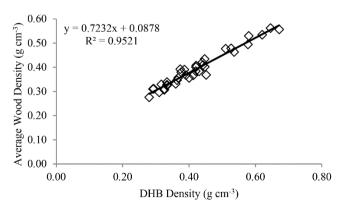
Figure 4. Correlation of average wood density of *Pinus taeda* by density the samples in 1.30 m height obtained.
